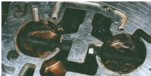
Picture J - Carburetor plates before P.i. treatment
